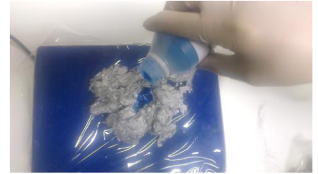
Fig. 11. 100 gram A component (pasta/vezel) met 20 gram B component (vloeistof).
